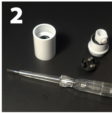
2 disassemble socket and find a flat screwdriver
