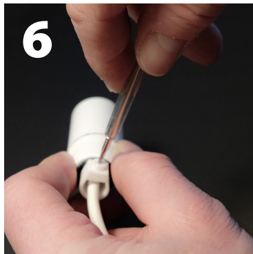
6 assemble socket and tighten cord grip screw
